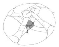
Lights will not operate until you remove the tab as shown (see drawing). Lights turn on when you move the UFO. Lights will stay on for 12 seconds once you stop moving the UFO.
